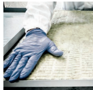
Positioning of the materials to be glued
