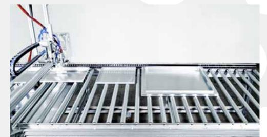
Example of robot for glue spreading on panels with or without edge
